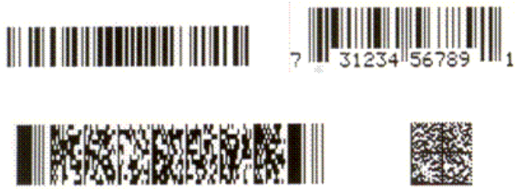
Figure 6 – Example of linear barcode and 2D symbology
