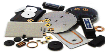
Figure 7 – Example of RFID tags
